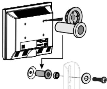
**CAUTION:** Verify adequate thread engagement with your screw **09**, washer **10**, spacer **11** combination AND TV/sound bar brackets.
