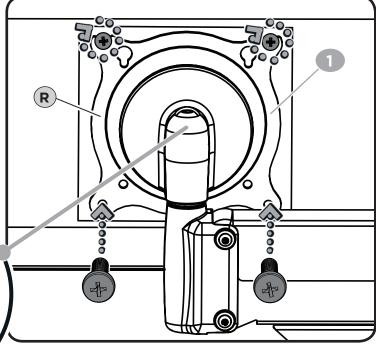
IMPORTANT: YOU SHOULD TEST THE TENSION OF THE ROTATING BRACKET R TO ASSURE THE MONITOR MOVES WITH EASE AND STAYS IN POSITION BEFORE TIGHTENING ALL SCREWS. See page 17 to adjust brackets tension.
