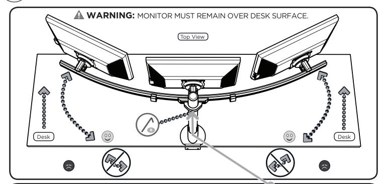
WARNING: DO NOT ATTEMPT TO ROTATE ENTIRE BAR WITHOUT LOOSENING SCREWS ON BACK OF MOUNTING BAR.
