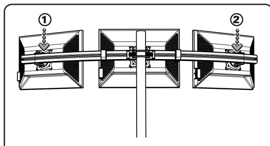
TIP: You can add spacers to the outside monitors to change the angle of the display. The below examples show the options for the array of monitors:
