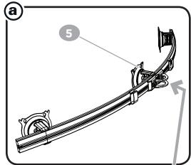
TIP: Loosen screws to where the bracket is loose enough to avoid scratching post.
